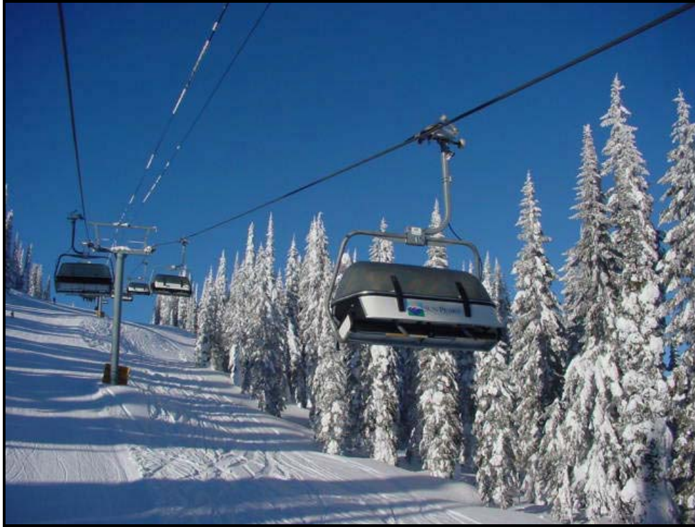
Sunburst Express Detachable Quadruple Chairlift with Bubble Cover (D4C-B)
